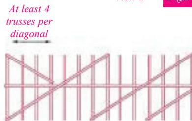
Two diagonals each end. One diagonal alternatively each side of centre line elsewhere
