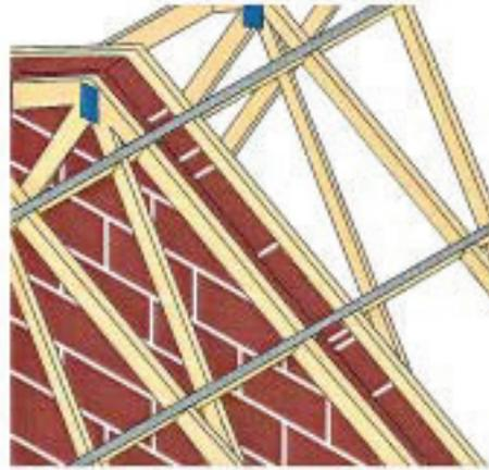
The Building Designer should ensure that, when required, adequate holding down fixings, 'C', are specified for both the trussed rafter and the wall plates or bearings.
