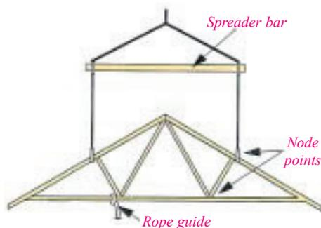
Where bundles of trusses are raised to roof level, caution should be exercised in the removal of the restraining bands (see section 3.11 figure 92). Should these bundles of trusses be stored either on a temporary working platform or at eaves level, the contractor should take the necessary steps to ensure that the supporting structure has sufficient strength and that a storage system as illustrated in either figure 90 or 91 is constructed.
