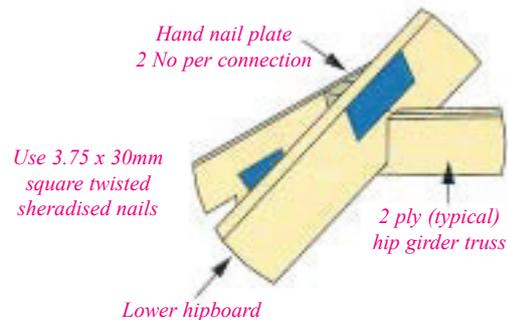
Hipboard to be notched over girder truss and butted together over centre of girder.
