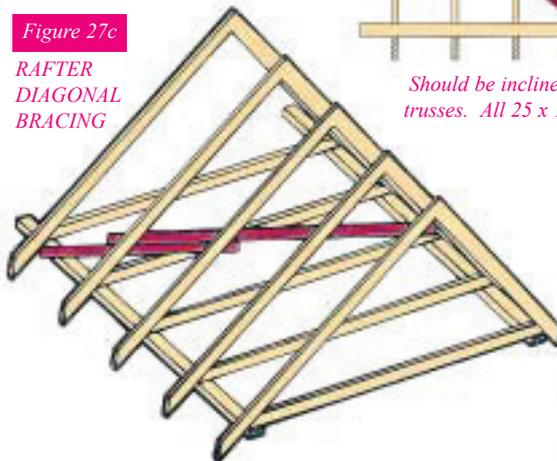
(One only shown and spliced) webs and all other bracing omitted for clarity. Braces to be 25 x 100mm free of all major defects and fixed with two 3.35 x 65mm galvanised nails at all cross-overs including wall plate. Braces to be inclined at approximately 45° to the tiling battens and repeat continuously along the roof.
