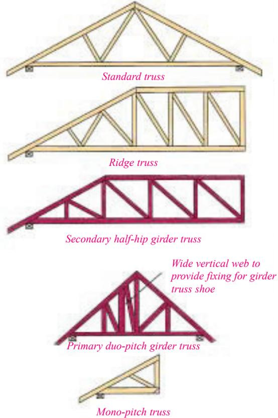
Wide vertical web to provide fixing for girder truss shoe
