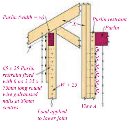
Purlin support post. Size 50 x (W + 25), extending to ceiling joint. Fix with one row of 4.0 x 100mm long round wire galvanised nails at 80mm centres for full length of post
