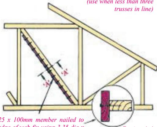
25 x 100mm member nailed to edge of web fix using 3.35 dia x 65mm long R/W galvanised nails, at 150mm centres.
