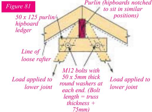
Max allowable load for this detail: 4.0Kn for C24
