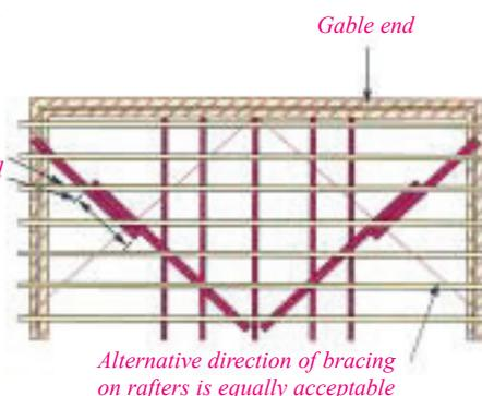
Immediately prior to the fixing of the permanent bracing and the tiling battens or sarking, all trussed rafters should be checked for straightness and vertical alignment. Whilst every effort should be made to erect trusses as near vertical as possible, the maximum deviations from the vertical shown in the following table may be permitted.
