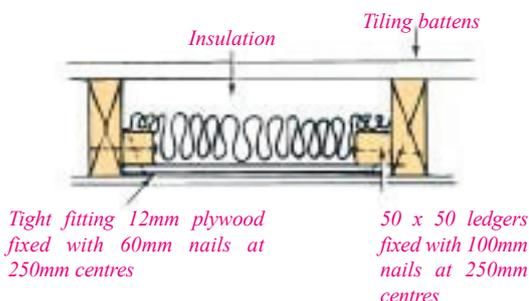
Tight fitting 12mm plywood fixed with 60mm nails at 250mm centres
