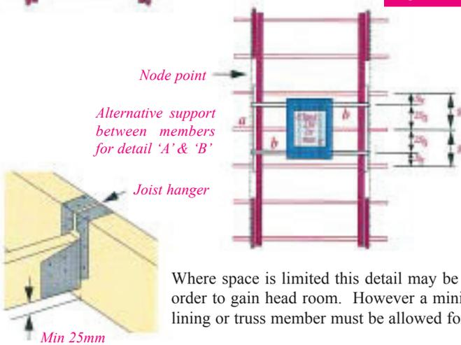
If water tanks are to be supported on the trussed rafters in accordance with the details shown then the provision for these must be taken into account at the design stage.
