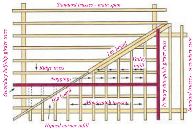
The roof is built up in the valley area using a mono-pitched valley set so that the half-hip girder carries the mono-pitch trusses and hipped corner infill, in the same way as at a hipped end. The span of the mono-pitch trusses is not generally greater than 3 metres and more than one half-hip truss may be needed between the ridge truss and the half-hip girder.
