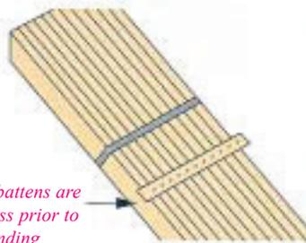
*Ensure that the battens are fixed to each truss prior to release of the binding*
