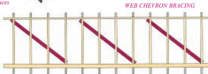
Should be inclined at approximately 45° (and each nailed to at least three trusses. All 25 x 100mm free of major defects and fixed with 3.35 x 65mm galvanised nails at all cross-overs.
